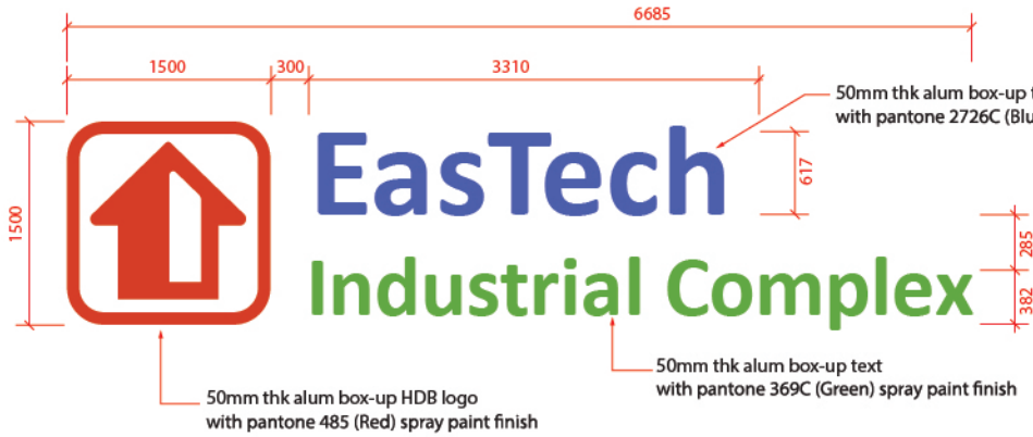
SIGNAGE TYPE 1 MOUNTED ON BUILDING FACADE (HIGH)
